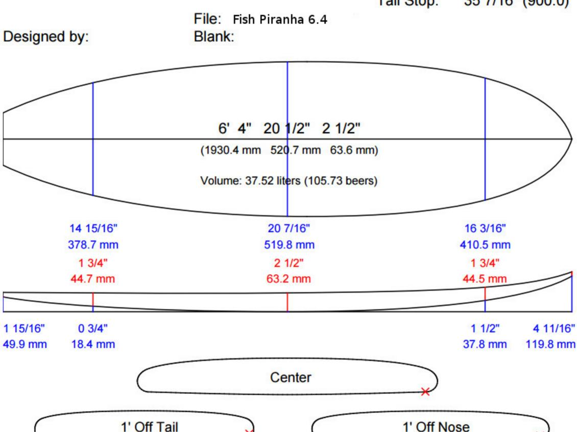
Measurements are center, one foot in and one foot back, over curve.
